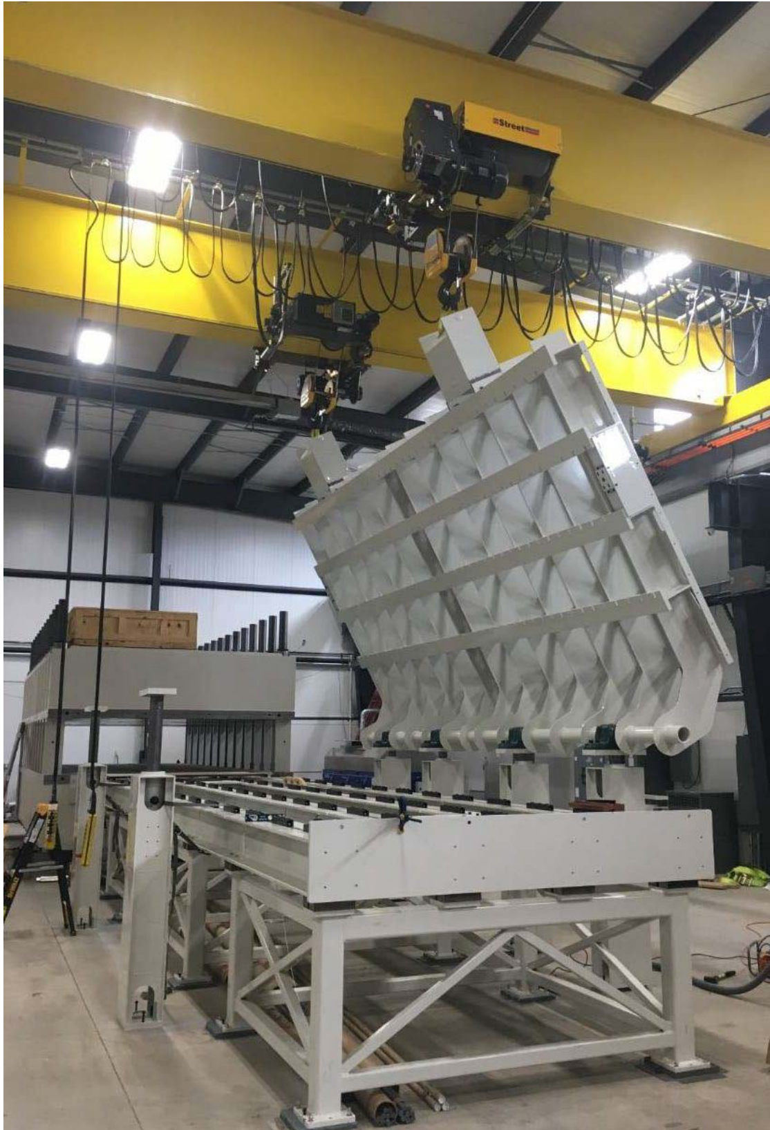
Figure 47. Picture of completed restraint with the die handling tooling in the open position
