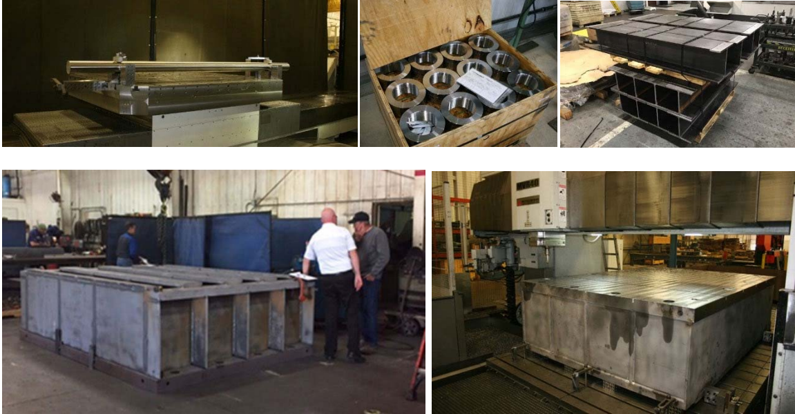
Figure 41. Pictures of the detail parts for the restraint during fabrication steps
