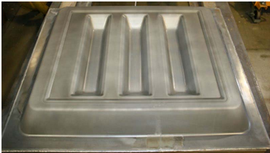
Figure 8. Formed aluminum consolidation bladder for the flat blade stiffened panels
