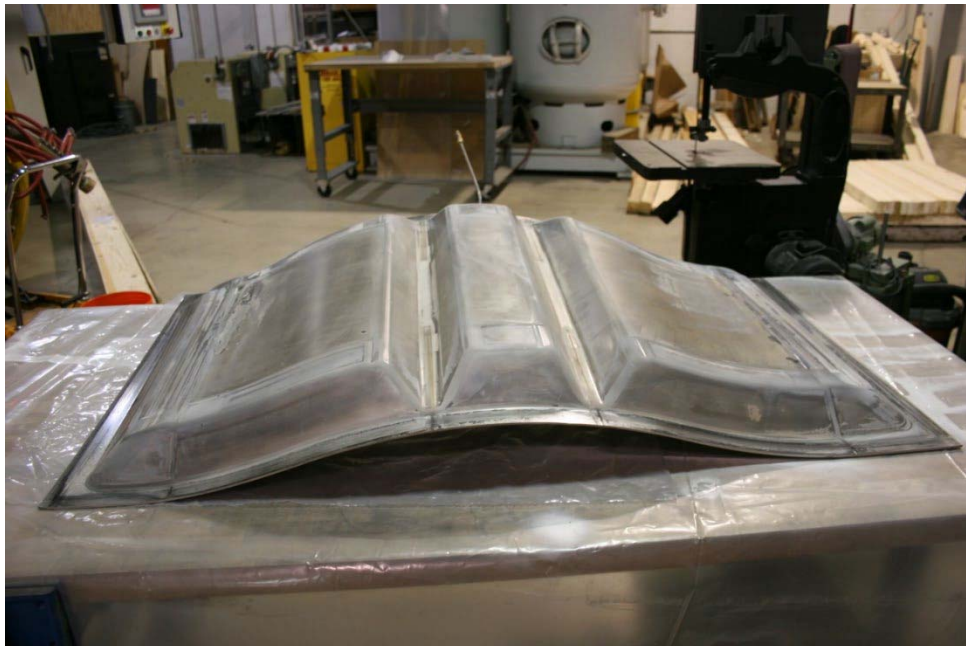
Figure 21. Formed aluminum bladder is now ready for co-consolidation of the stringers to the complex contour panel
