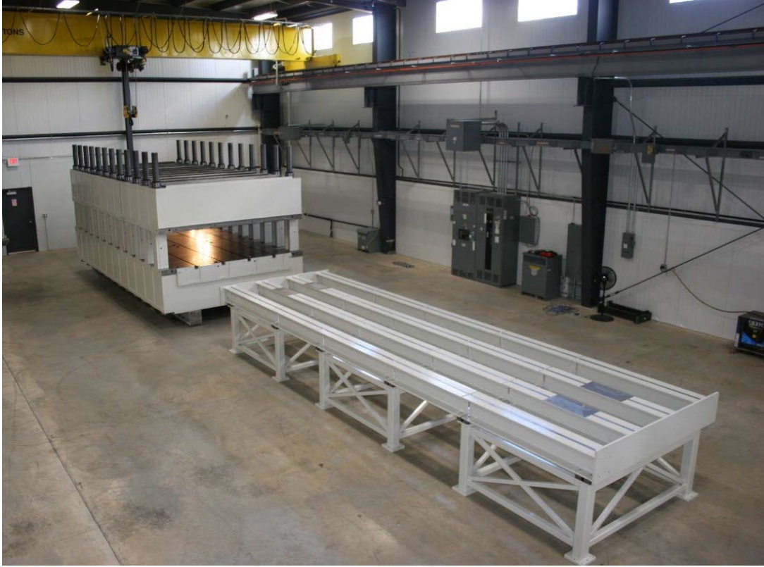
Figure 45. Picture of completed restraint with a portion of the die handling tooling installed
