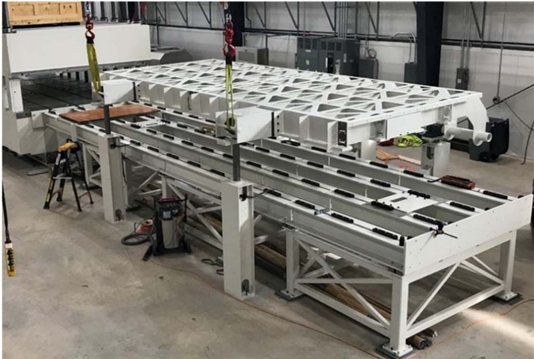
Figure 46. Picture of completed restraint with a portion of the die handling tooling installed
