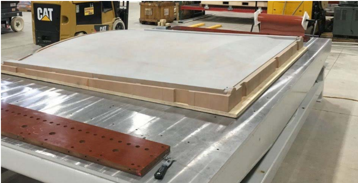
Figure 59. Picture of a machined casting mandrel for one of the tool modules
