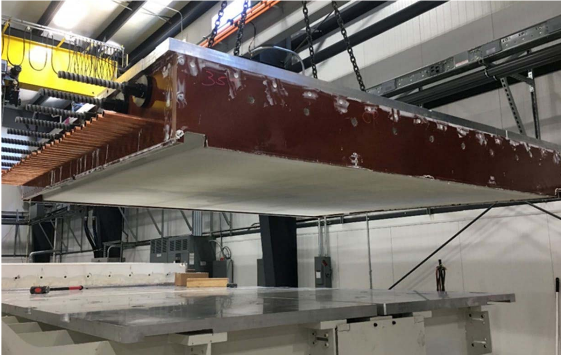
Figure 66. Picture of cast tool section being transported to the tool handling fixture to be installed and readied for processing trials
