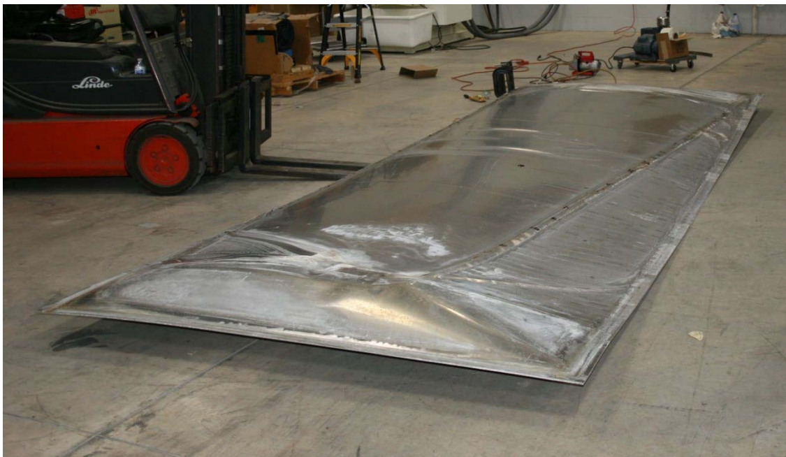
Figure 78. Forming of the bladder was completed plus this processing run validated the capability of the system to heat and apply pressure
