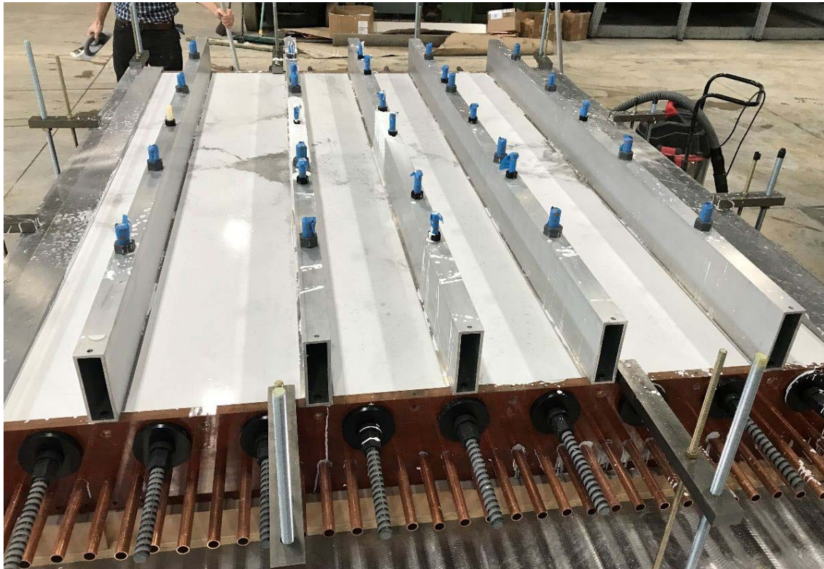
Figure 65. Picture of tooling section after casting of the Ceradyne 120 material
