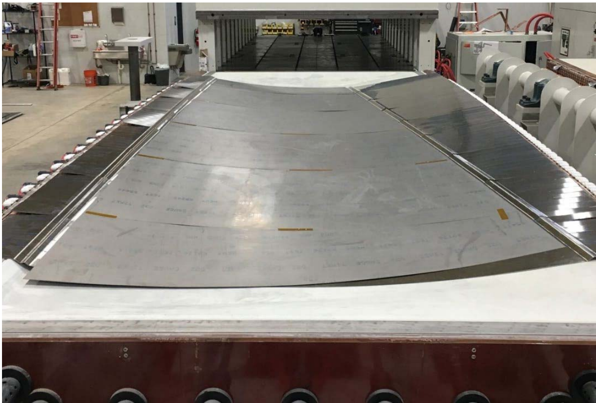
Figure 72. Picture of titanium caul sheet placed on the surface lower tool
