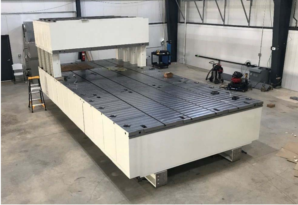
Figure 43. Placement of the first upper restraint element
