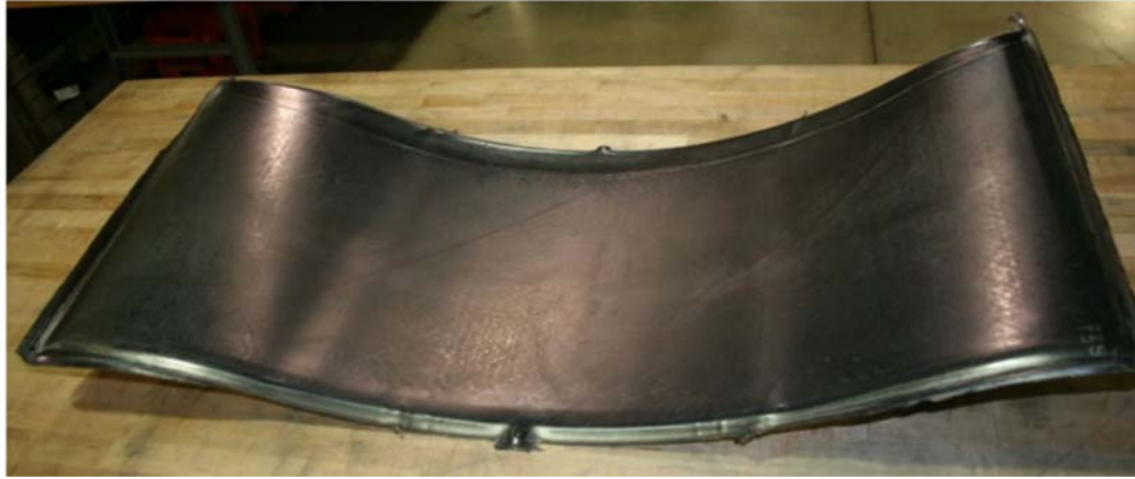
Figure 18. Formed aluminum bladder for induction consolidation of complex contoured thermoplastic skin
