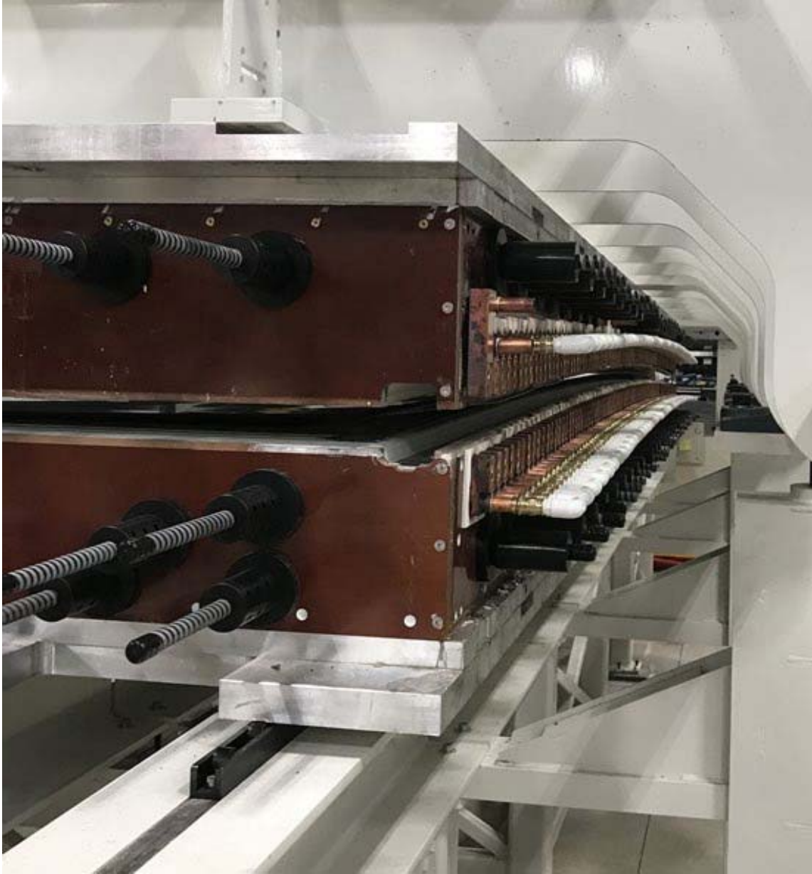
Figure 70. Depiction of the upper and lower tool halves placed together and ready to be loaded into the restraint
