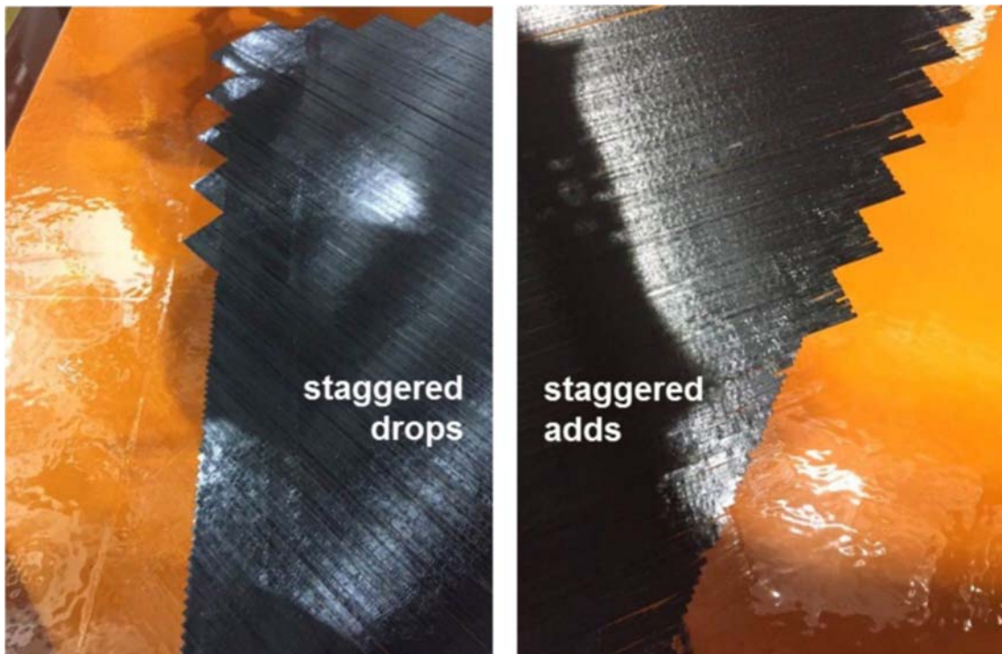
Figure 26. Examples of staggered adds and drops need for tailored lay-ups
