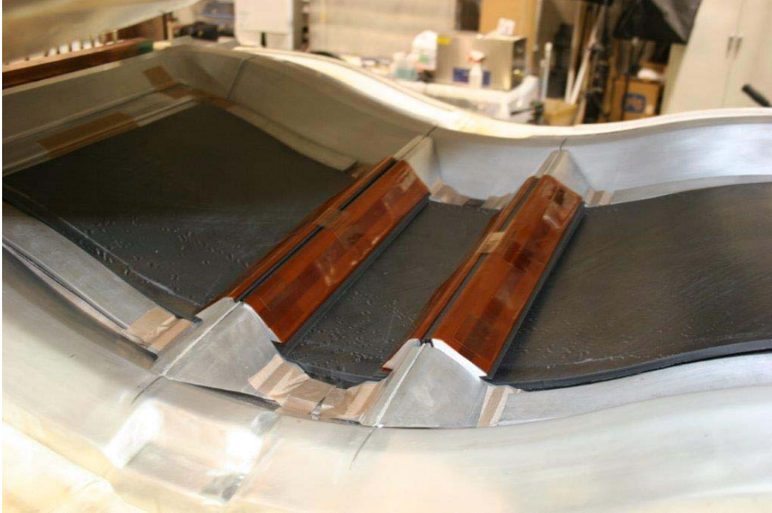
Figure 22. Set-up for the co-consolidation of the stiffened panels
