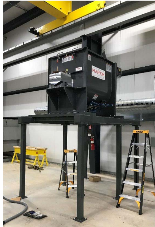
Figure 64. Depiction and picture of the ceramic mixer and tool casting system
