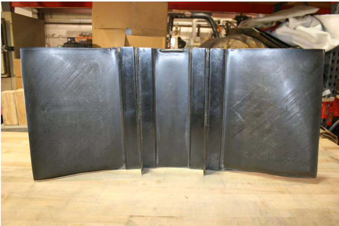
Figure 23. Finished co-consolidated blade stiffened complex curvature component
