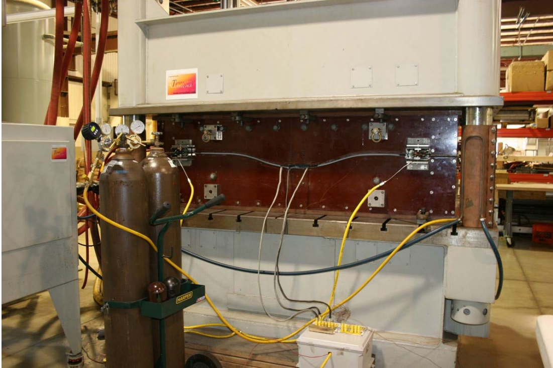
Figure 16. Induction consolidation processing system set-up for part fabrication cycle
