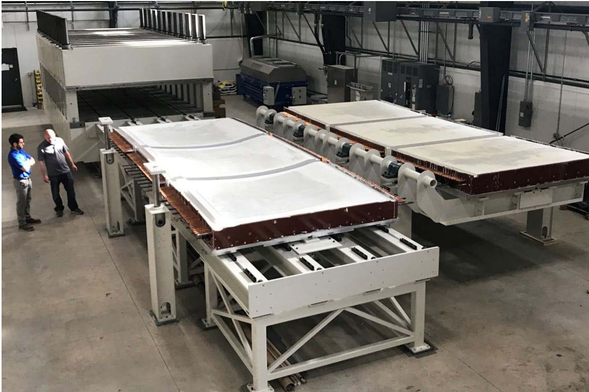
Figure 68. Picture of tool handling fixture with all six tooling sections loaded and assembled
