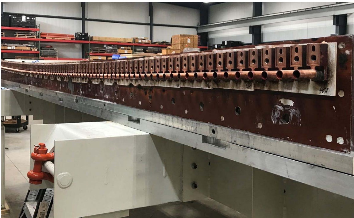
Figure 69. Picture of copper coil connectors after brazing
