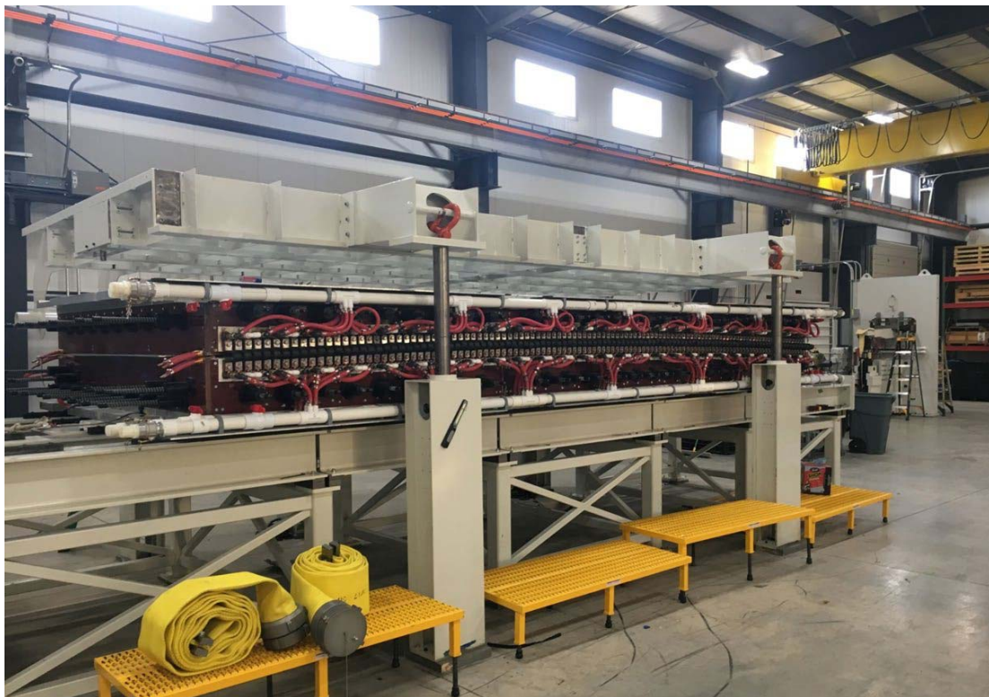
Figure 76. Picture of the upper tooling rolled over in preparation for forming of the bladder
