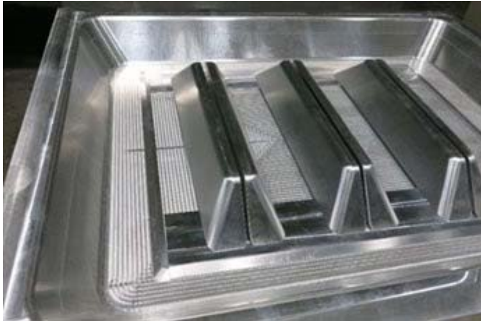
Figure 9. Machined aluminum co-consolidation tooling
