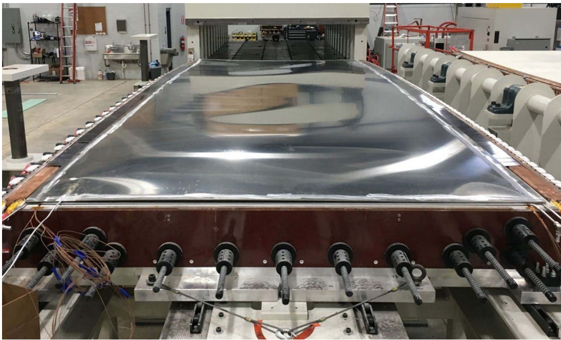
Figure 74. Picture of the unformed aluminum bladder placed on the lower tool with the lower smart suscepter, titanium caul, and simulated part (aluminum sheets)
