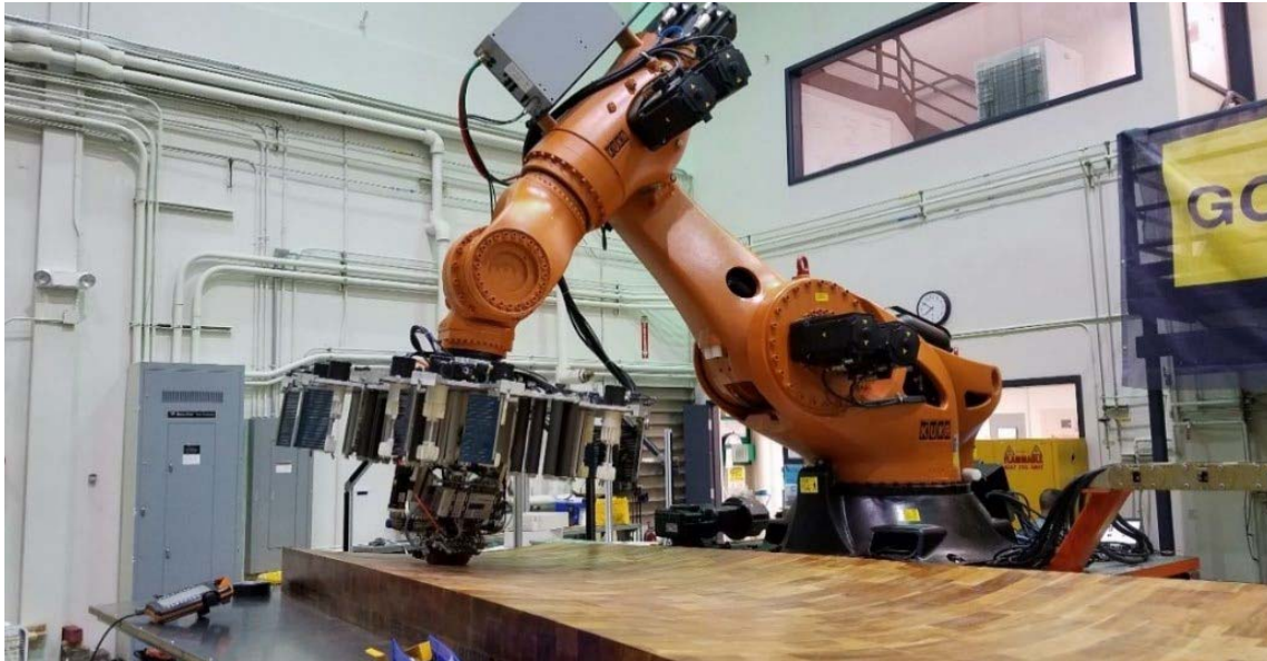
Figure 53. Picture of ½" wide tape head installed onto the robot performing a mechanical test showing tape laying course travel over the demo skin lay-up tool
