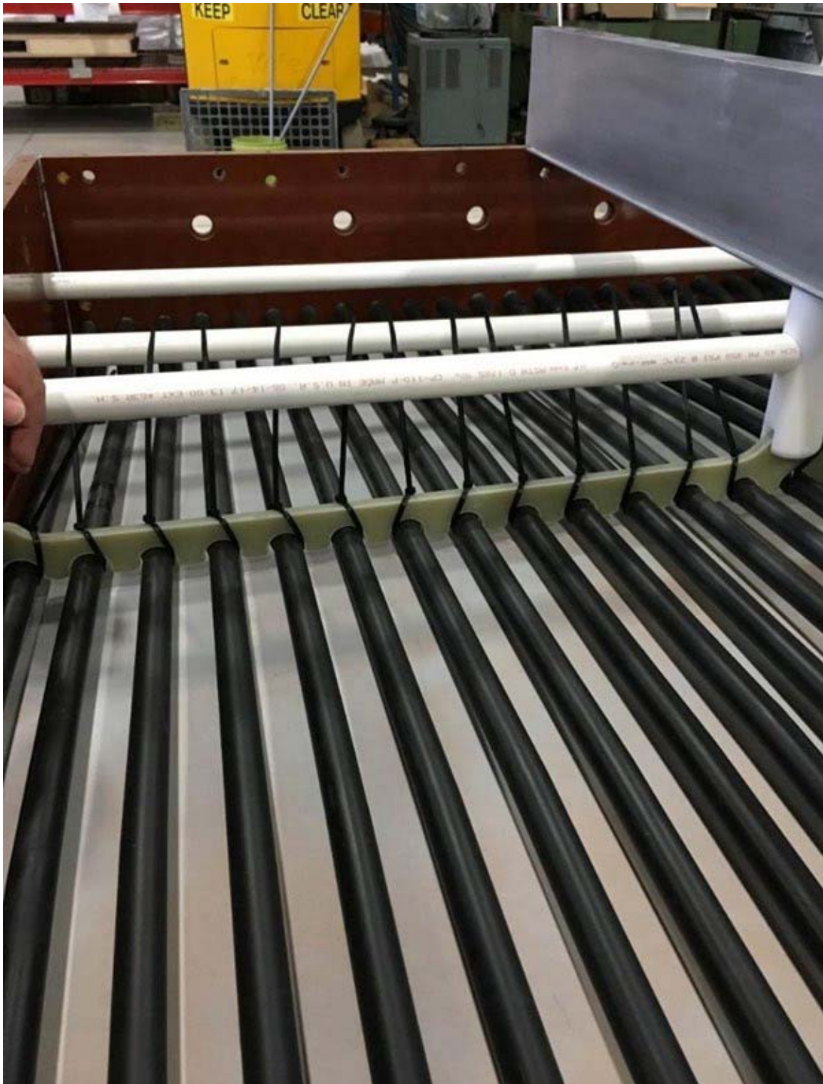
Figure 61. A picture of the secured coil segments located in the tool assembly build-up prior to casting of the Ceradyne 120 material
