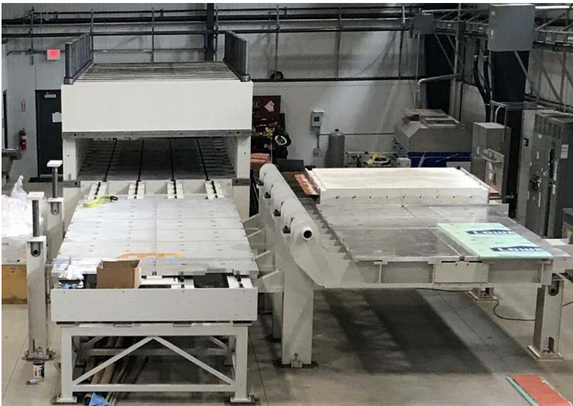
Figure 67. Picture of tool handling fixture with the first cast tool section loaded
