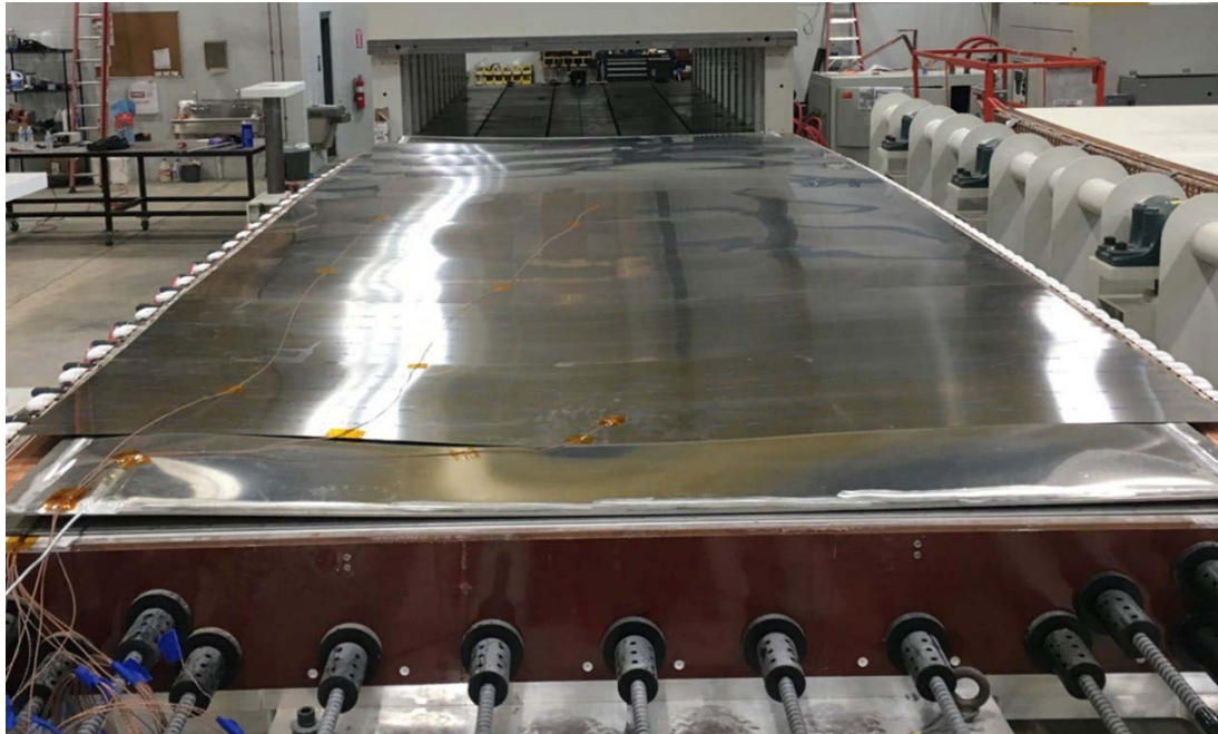
Figure 75. Picture of the upper smart susceptor placed on the tool which completed the stack-up of the internal components needed to form the bladder
