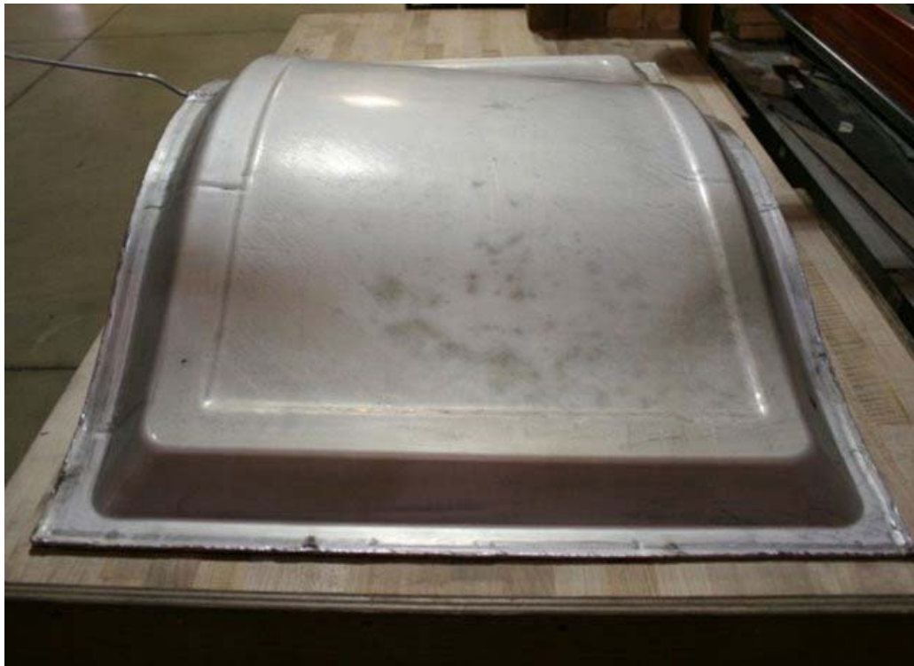
Figure 17. Formed aluminum bladder for induction consolidation of complex contoured thermoplastic skin
